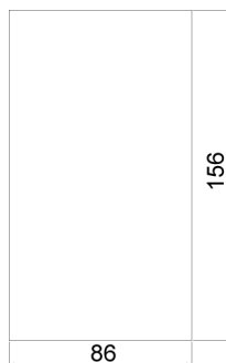
Fig. 3-5: Hole dimension of operating panel
